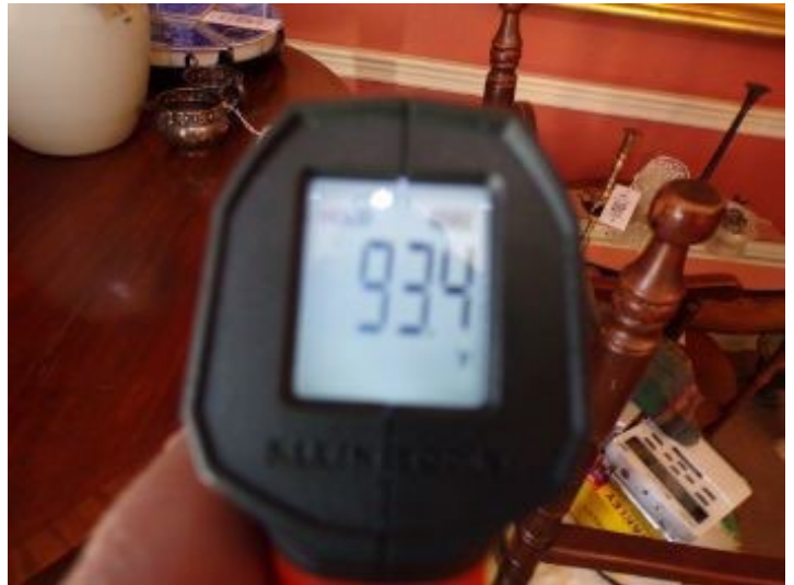
93.4 degree supply air heat
