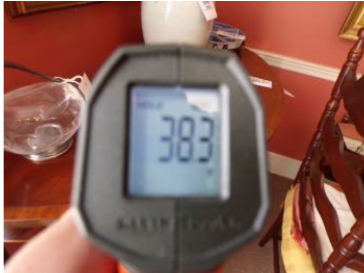
38.3 degree supply air cool
