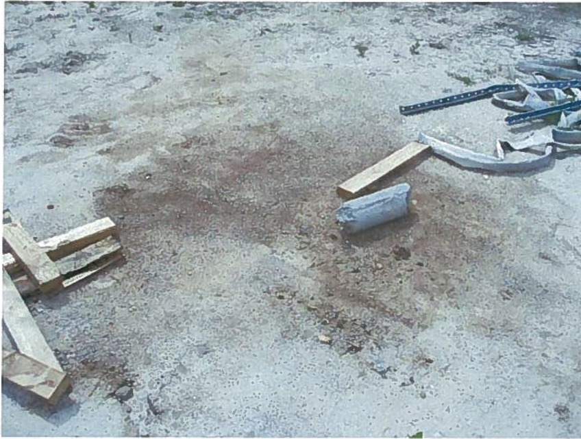
Photo 15: Small area of visually impacted soil at the former drum storage area.
