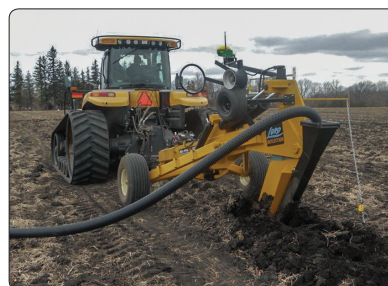
Top: Pattern tiled field. Left: Trenching tile has a capacity of approximately 1,000 feet per hour. Right: Plowing tile increases the capacity to 3,000-4,000 feet per hour.
