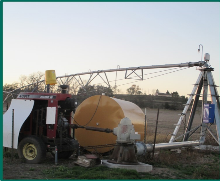
Pivot with Motor Well & Diesel Tank
