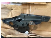
#68 • Hood hinge set. Moisture damage
