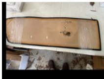
#25 • Standard door panels (pair) Moisture damage as seen in picture
