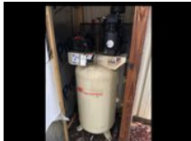
#273 • Ingersoll Rand Air Compressor It is a 2stage /230-volt single phase 80 gal. with no known issues. Approximately 4 years old
