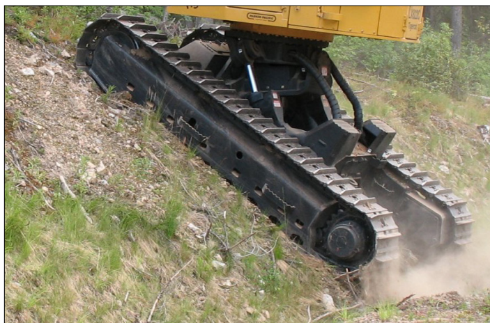
R7-150L-2 Tigercat FH400 undercarriage with long track frames and wide stance for excellent stability on slopes.
