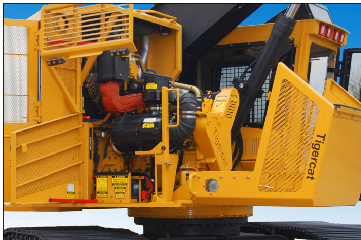
Easy access to daily service points with hydraulically retracting engine hood enclosure.
