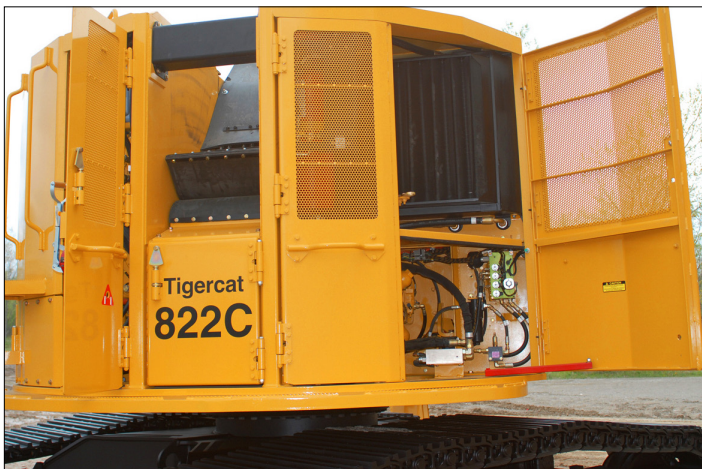
Clear access to the pumps; Cooling air is drawn from the rear, away from the saw discharge area.
