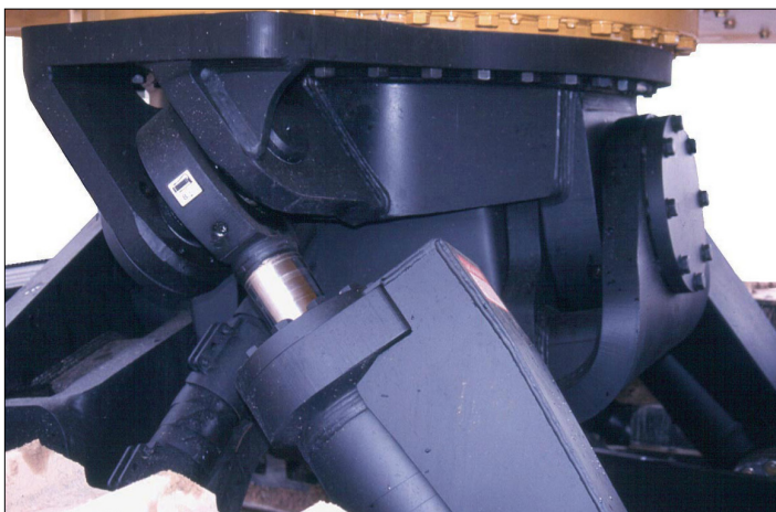
Super-duty leveling system constructed with thick steel plate, massive pins and cylinders.
