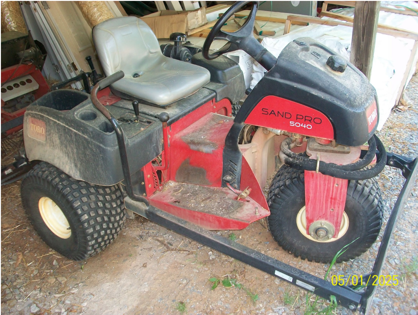
LOT 6 — Toro 5040 Three Wheel Sand Rake, SN #08705; 3 wheel drive, hydrostatic drive, 18 hp Vanguard 4 cycle engine, rear grooming rakes, front blade for pushing or leveling, 2306 hours
