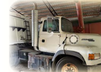
1996 Ford AeroMax L9000 Semi Truck. Day Cab Twin Screw Cummins Engine 9-Spd Transmission
