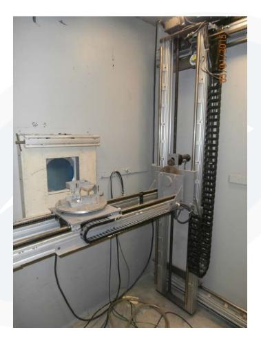
The motions are motorized and are controlled by 90VDC Variable Motor Controllers that can be purchased easily in the USA. The Axes are as follows:
