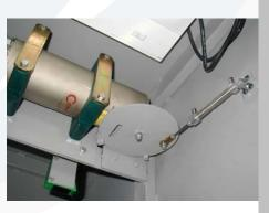
The Tube Shutter of the NX-CIS160-LDA System as seen from the Maintenance access door.
