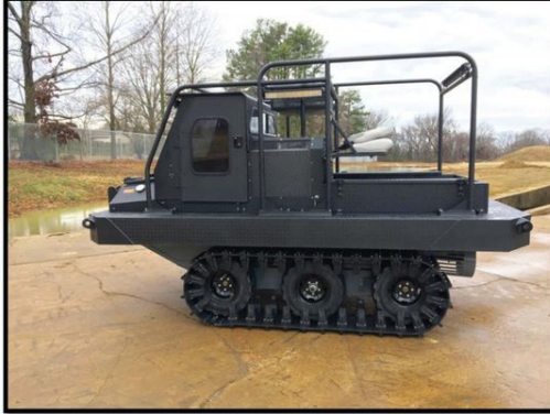
XTB66 BASE UNIT 6 x 6 TRACKED AMPHIBIOUS UNIT WITH WATER PROPULSION
