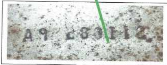
OEM correct primary confidential VIN is on the upper radiator support
