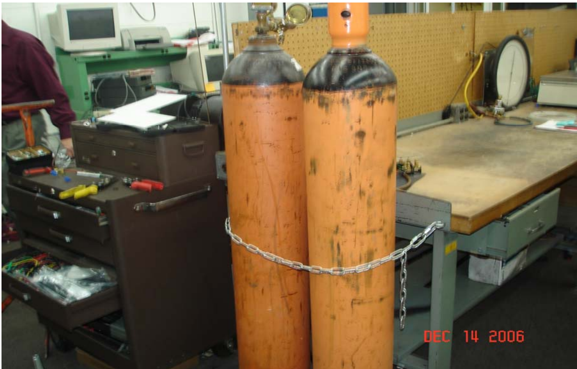
Properly stored tanks
