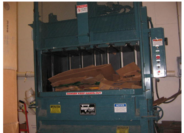
Photo #6: Cardboard compactor
