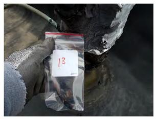
**Photo #8** Sample 13, sealant on condenser piping on main roof.
