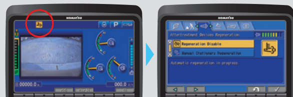
Aftertreatment device regeneration screen
