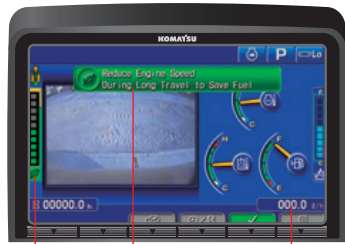
Ecology gauge Fuel consumption gauge Ecology guidance
